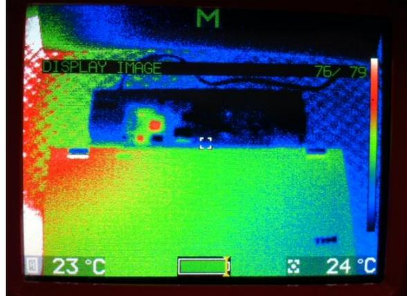
Figure 42: Thermal image of dock + laptop (with implant)
