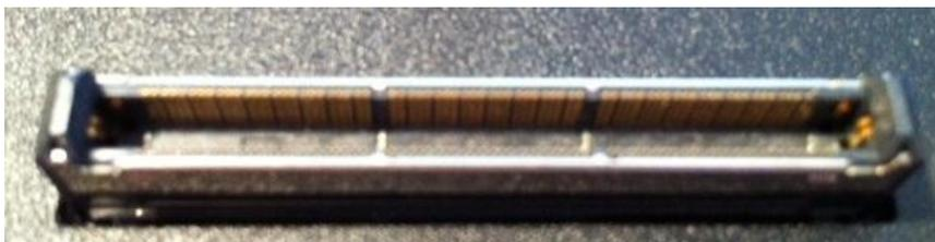
Figure 28: Dell E-series proprietary dock connector
