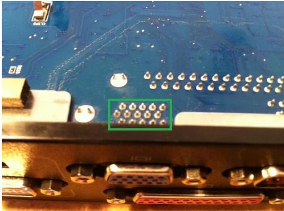
Figure 20: VGA connector pins
