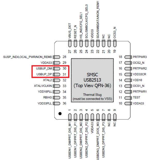
Figure 27: Hub controller chip pin-out in datasheet
