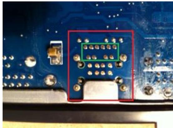
Figure 14: The module pins on the PCB
