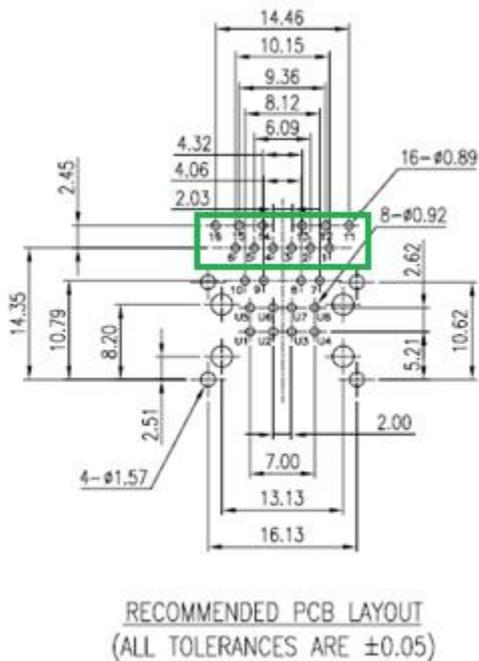
Figure 15: Ethernet pin locations
