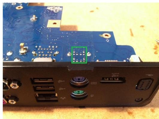
Figure 23: PS/2 module PCB pins
