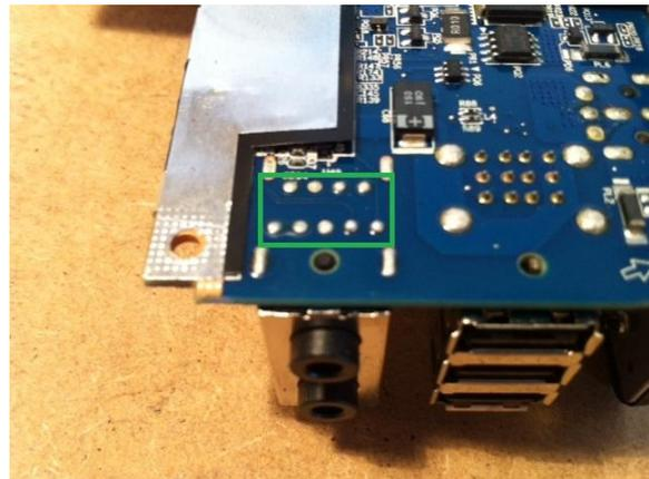
Figure 25: Audio module PCB pins
