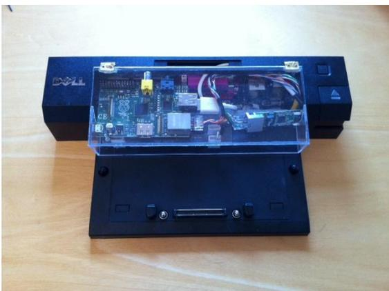
Figure 37: Spy-Pi implant installed in a Dell PR02X
