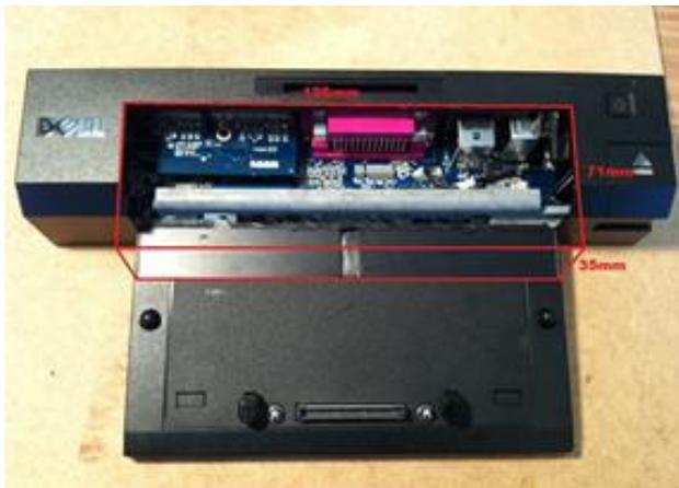
Figure 34: Docking station with cover removed
