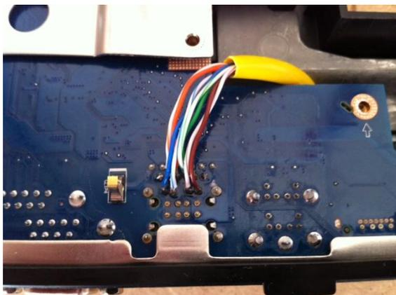
Figure 17: Connected Ethernet tap
