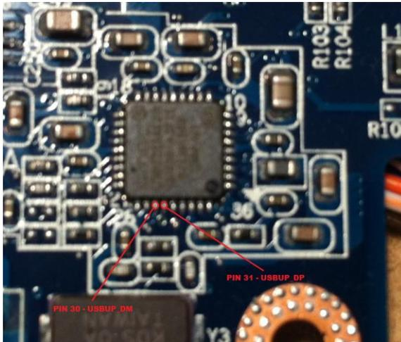
Figure 26: Hub controller chip upstream hub connections
