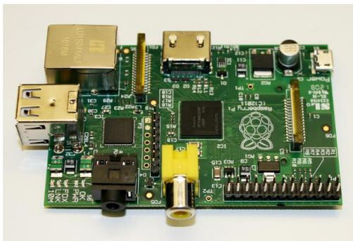
Figure 30: Raspberry Pi Model B
