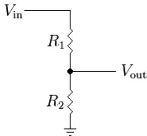
Figure 36: Simple voltage divider circuit
