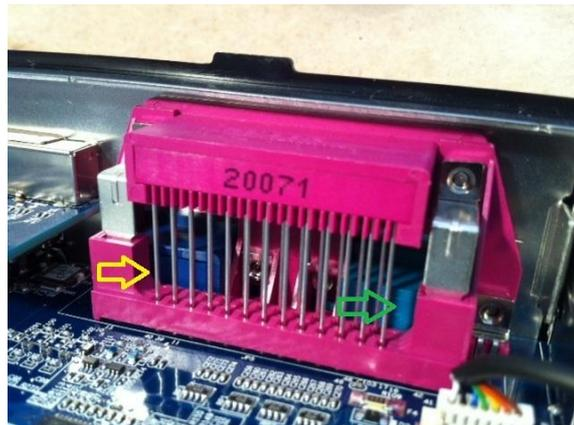
Figure 21: VGA connector hidden behind a cage of pins
