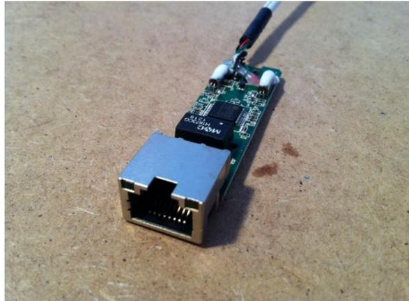
Figure 32: USB Ethernet adapter
