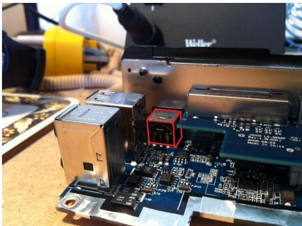
Figure 35: Rear of the main DC power input connector
