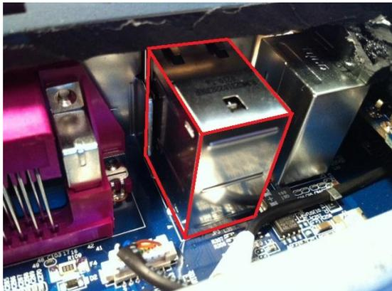
Figure 13: Combined Ethernet / 2 x USB module
