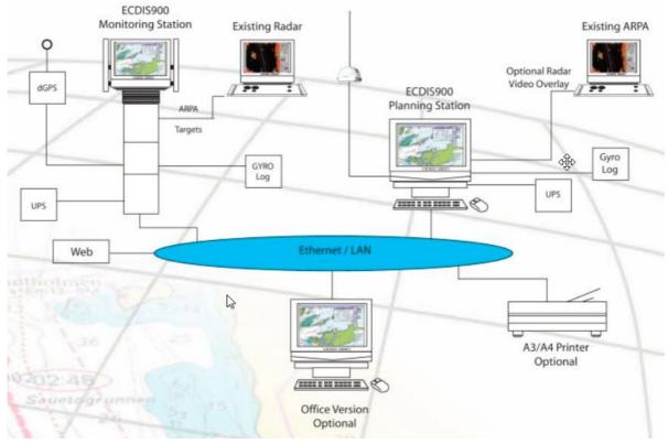
Figure 1: Diagram of systems typically connected to a ship's LAN [source http://pdf.nauticexpo.com/pdf/maritime-information-systems/ecdis-900/31325-42061-\_9.html]
