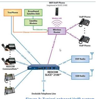
Figure 3: Typical onboard VoIP system [source http://www.redcom.com/markets/shipboard-communications/]
