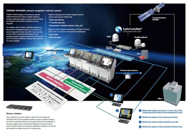
Figure 2: Onboard navigation network system [source http://www.furuno.com/en/business\_product/merchant/product/voyager/]
