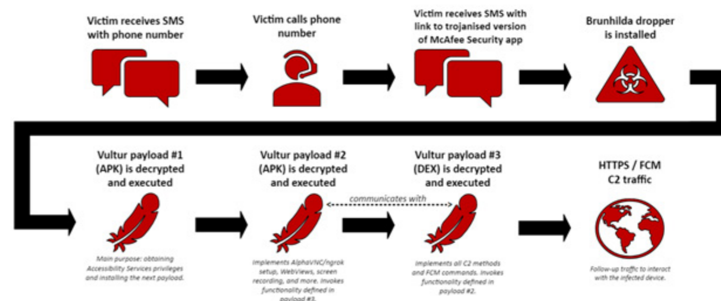
Figure 4: Visualisation of the complete infection chain. Note: communication with the C2 server occurs during every malware stage
