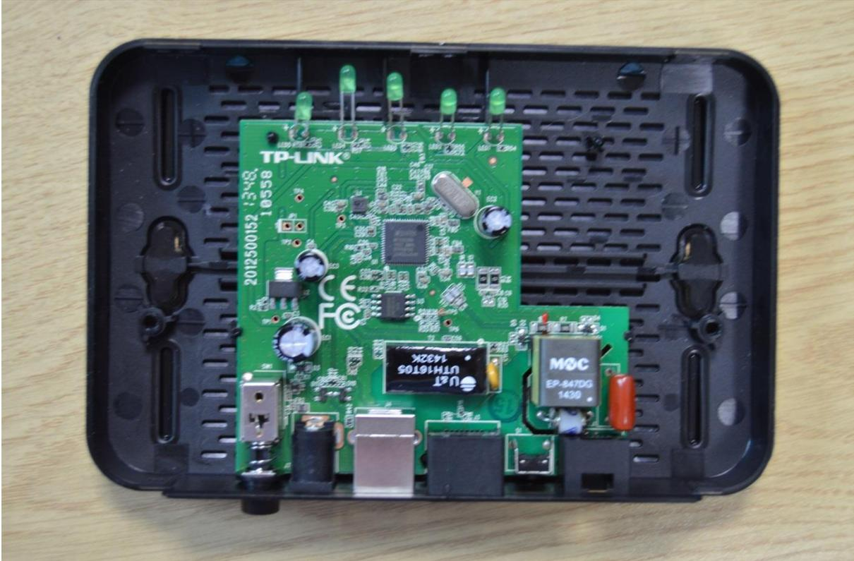
Carefully pull the back of the board up then pull it away from you (aka away from the back of the router and the plastic casing for the buttons). You should now be left with the board itself:
